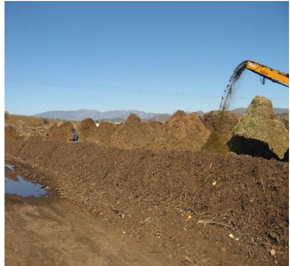
Photo 6.58: Windrows of compost at Robertson Composting Facility
