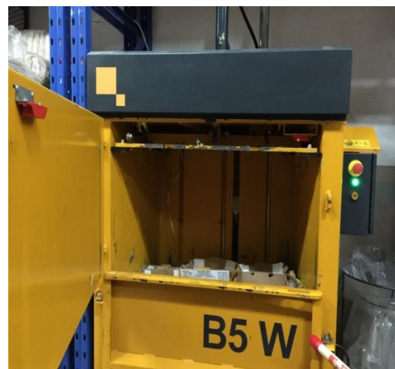
Photo 6.2: Cardboard compaction at Robertson Spar
