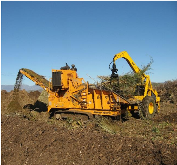
Photo 6.57: Hired chipper for Robertson Composting Facility
