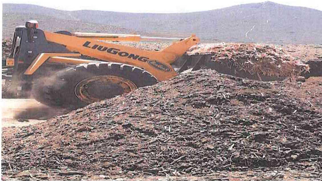
Figure 3: Wood chips used to cover waste
