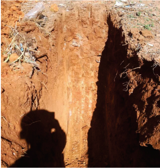
Figure 6: Typical orange alluvial soil exposed in test pits
